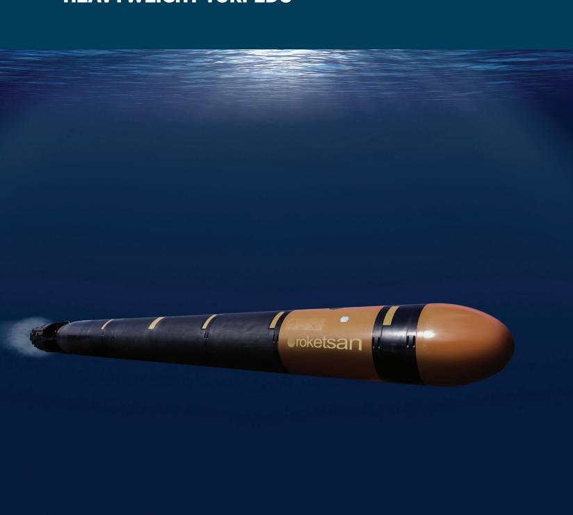
**AKYA** is a fully indigenous design, new generation Heavyweight Torpedo launched from submarines to engage submarines and surface targets of various types. AKYA is a high speed, long range, fully autonomous or fibre optic wire guided torpedo with active/passive sonar homing head, In addition, AKYA employs wake homing guidance for surface targets.
