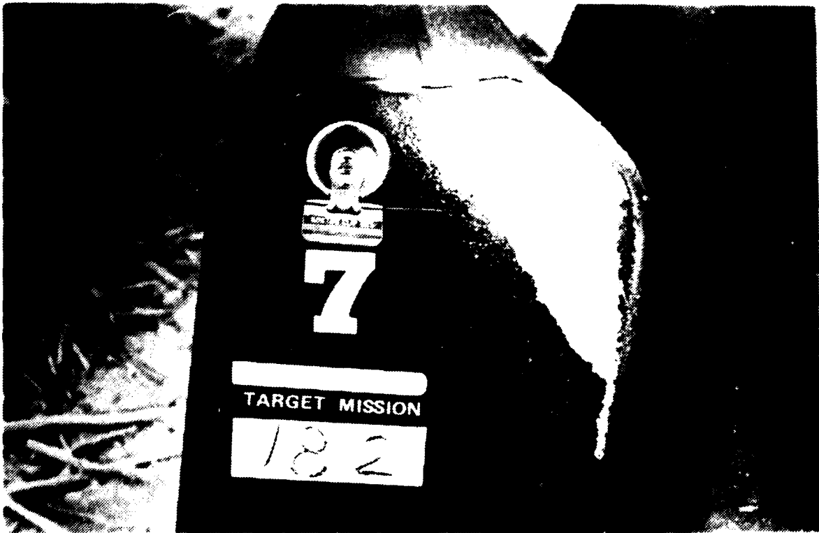
Fig 18. Perforation of Fuel Can Simulating Bow Fuel Tank, Impact 17, Mission 2, Target 18 (NOTE: This impact is mis-numbered and should read 17.)
