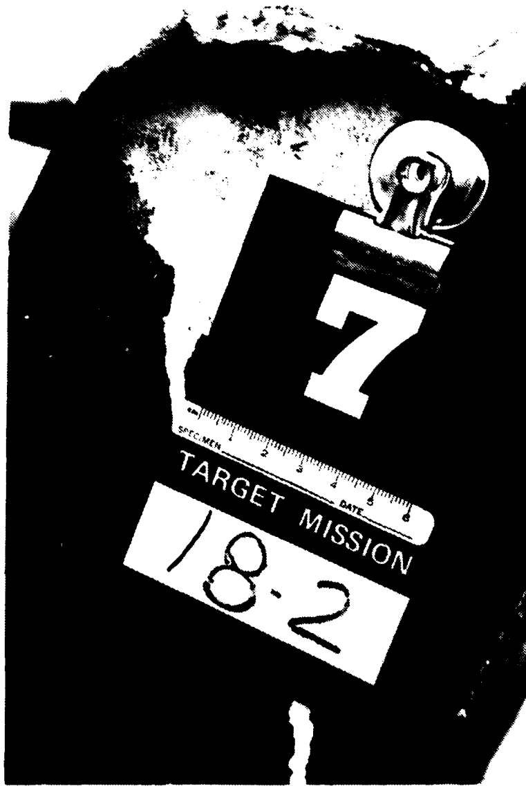
Fig 20. Perforation of Fuel Can Simulating Bow Fuel Tank, Impact 17, Mission 2, Target 18 (NOTE: This impact is mis-numbered and should read 17.)
