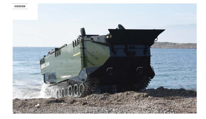
The Marine Assault Vehicle (MAV) is the latest technology amphibious vehicle designed by FNSS to meet amphibious operational requirements.
