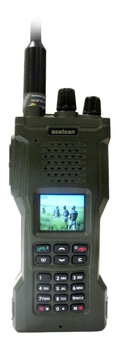
PRC-5433 is a new generation Software Defined Networking Radio (SDNR) that is designed to provide high speed data communications for the user in the tactical field. A wide operating frequency spectrum bandwidth of 30-512 MHz and high level Electronic Warfare Protection features provides much more field maintenance ability to PRC-5433.
